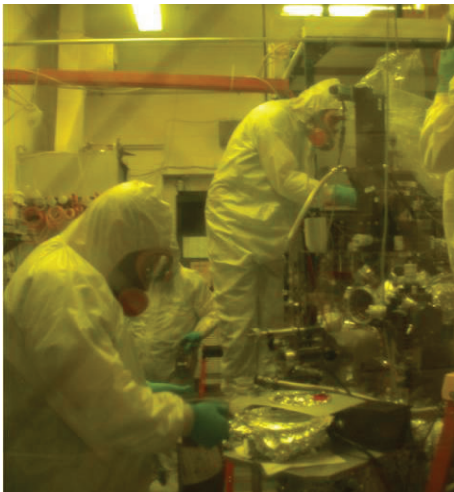
Figure 7. LPLS hotjob 2012 (r to l) Dave Moore (MST-16), Tomasz Durakiewicz, and John Joyce. A hot job is considered an exclusion area while work is being performed and has the potential for radioactive release. Special personal protective equipment is required such as full face respirator, fabric and paper clothing, and gloves taped to footwear.
