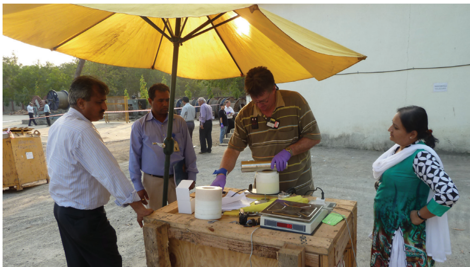
Figure 4. Source encapsulation in special form capsule (ONGC).
